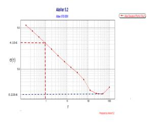
Figure 18. Allan deviation plot for Sandia 14 pin accelerometer
