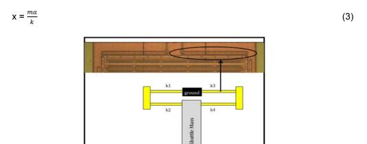
Figure 3. Sandia Capacitive MEMS accelerometer structure [6]
