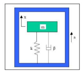
Figure 2. Sandia Capacitive MEMS accelerometer structure [6]
