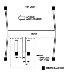
Figure 7. Movement of fingers when acceleration is applied [5]
