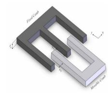
Figure 9. Electrode movements of comb-fingers [6]
