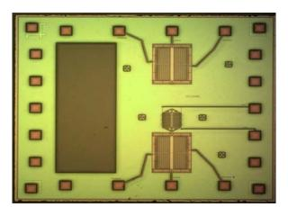
Figure 1. Sandia Capacitive MEMS accelerometer structure
