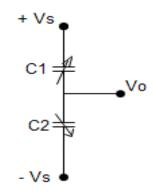
Figure 8. Circuit Model for Capacitive Voltage Divider [7]
