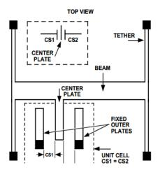
Figure 6. Capacitive fingers at rest [5]
