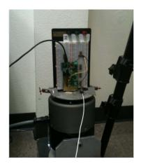
Figure 16. Test set up for Vibration test
