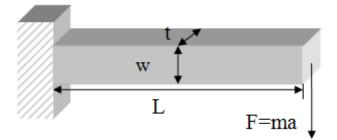
Figure 4. Cantilever beam movement with one rolling beam end [5]
