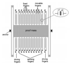
Figure 5. Capacitive interaction between movable and fixed fingers [5]
